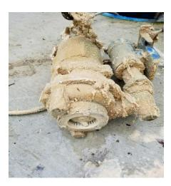
The image to the left of the discharge sewage pump is the impact of patrons not abiding by the grease disposal policy outlined in the reservation form. Failure to abide by the policy with eventually result in the main sewage line being blocked rendering the campground with no sewer discharge for the days it would take to clear the line of the blockage.
