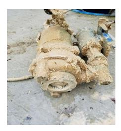
The image to the left of the discharge sewage pump is the impact of patrons not abiding by the grease disposal policy outlined in the reservation form. Failure to abide by the policy with eventually result in the main sewage line being blocked rendering the campground with no sewer discharge for the days it would take to clear the line of the blockage.
